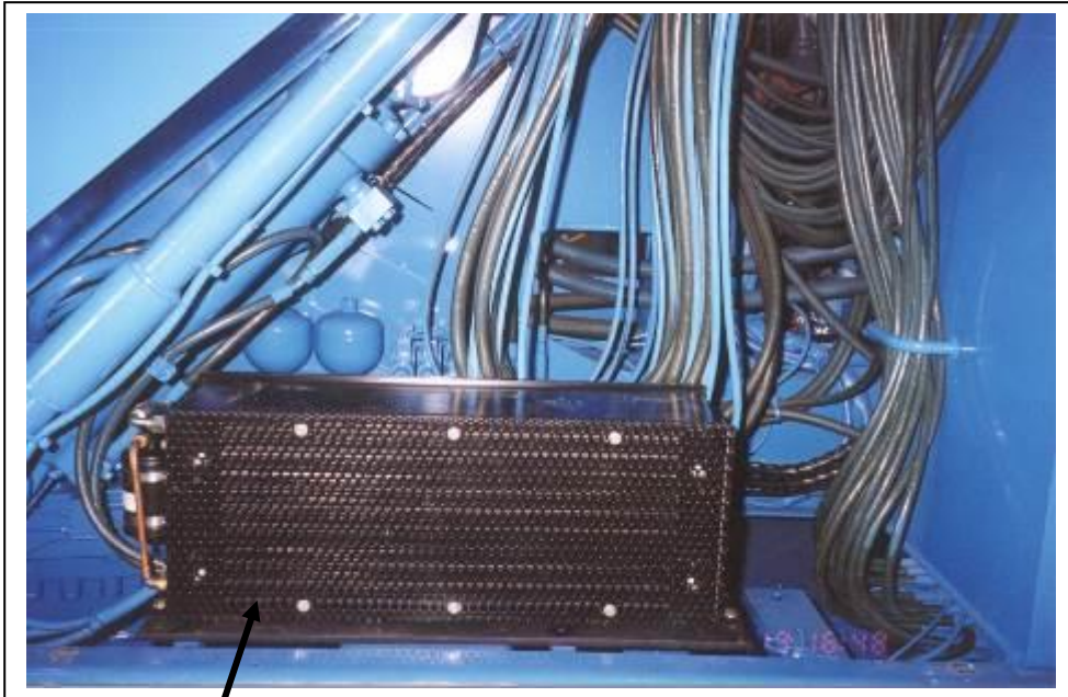
Condenser in place
